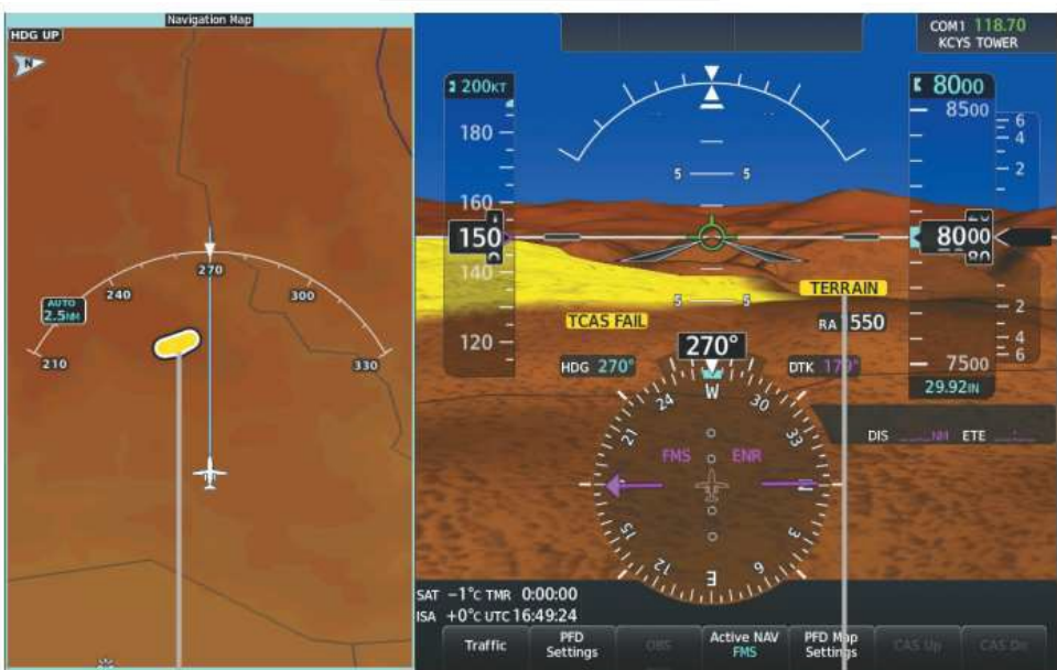
Potential Impact Area (Navigation Map and PFD with Synthetic Terrain enabled)
