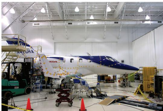
Fig. 26 Ground-vibration test.
