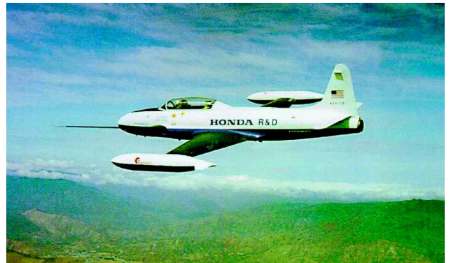
Fig. 3 T-33 aircraft modified for NLF flight test.
