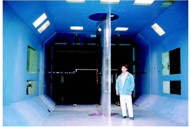
Fig. 2 Actual wing structure in Honda low-speed wind tunnel.
