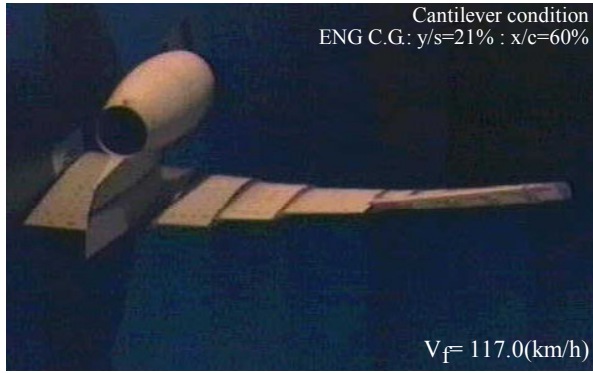
Fig.18 Low speed wing flutter test
