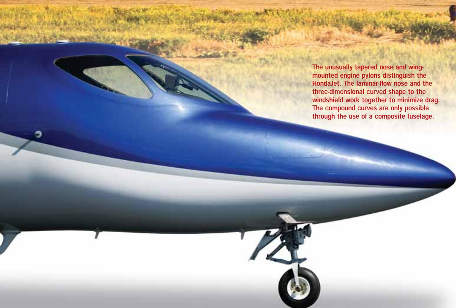
The unusually tapered nose and wing-mounted engine pylons distinguish the HondaJet. The laminar-flow nose and the three-dimensional curved shape to the windshield work together to minimize drag. The compound curves are only possible through the use of a composite fuselage.
